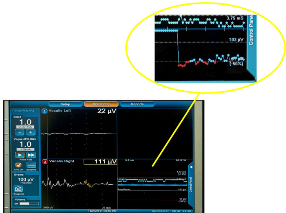
Fig. 2 The NIM ® -Response 3.0 in the APS ™ setting. Please notice the recorded “event” (yellow circle), as opposed to the neural activity prior to the “event” (big screen)
